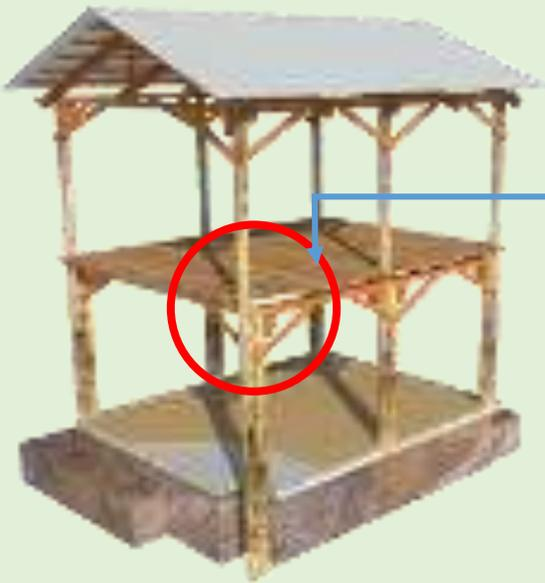
Knee bracing shall be provided each connection between posts and beams.
