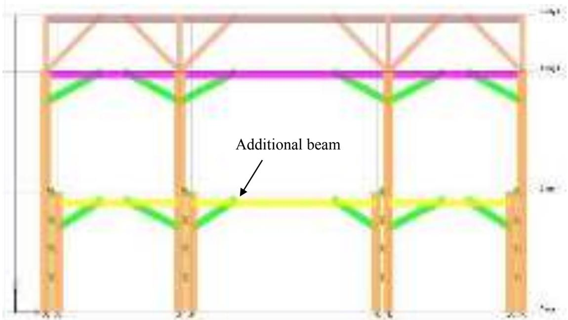
Figure 3: Additional beam below the level of existing beam
