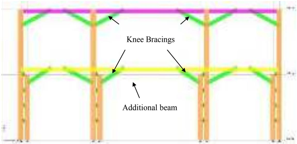
Figure 2: Additional beam above the level of existing beam
