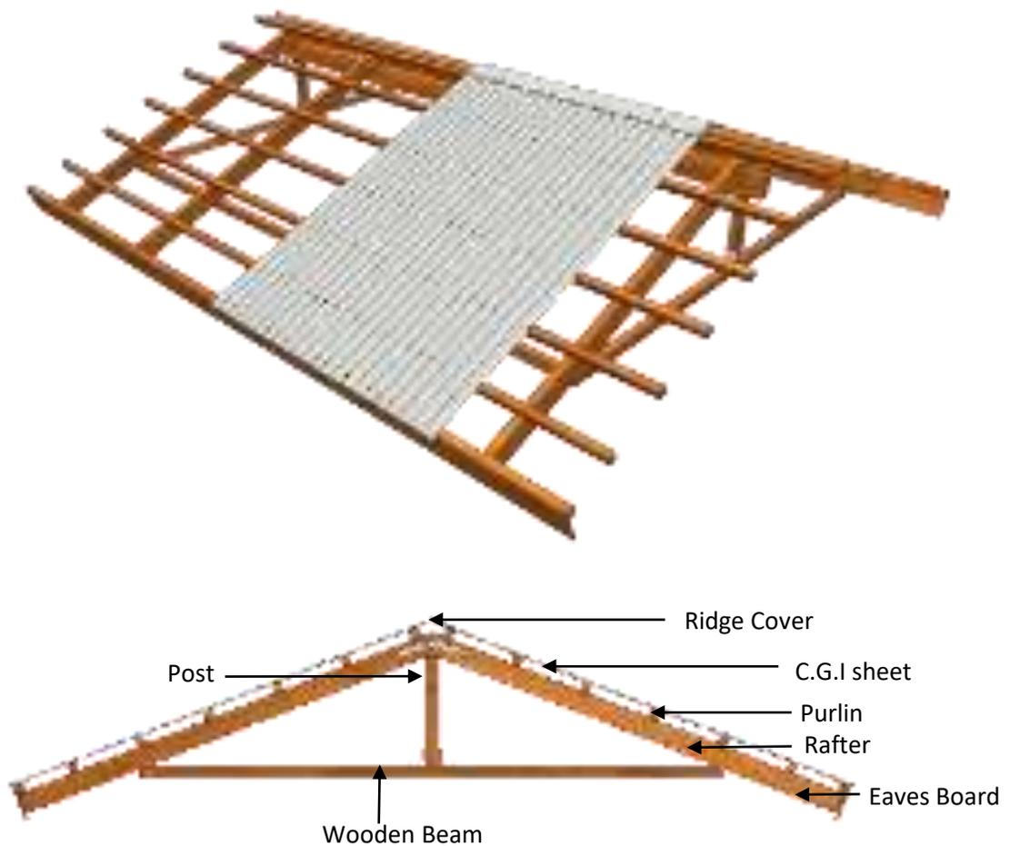
A **timber roof truss** is a structural framework of timbers designed to bridge the space above a room and to provide support for a roof. Trusses usually occur at regular intervals, linked by longitudinal timbers such as purlins. Rafters are inclined timbers fixed between wall plate and ridge which transmit live and dead loads to wall plate.
